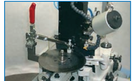
Fast saw blade tensioning system
